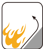
Reduced Fire Propagation NF C32-070-2.2(C1) IEC60332-3-24 EN50266-2-4
